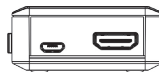
DC 5V (Micro USB power input)
